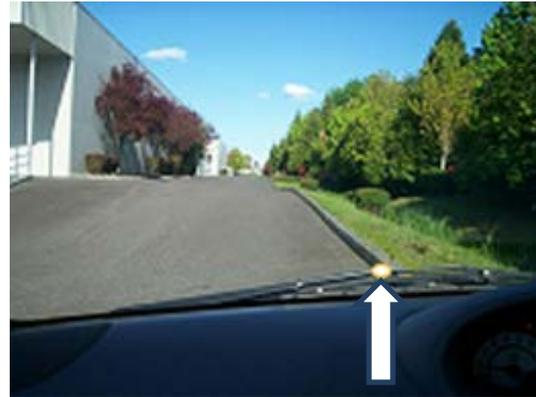
This round sticker tells the driver to line the sticker up with the curb to ensure the wheels will be about one foot from the curb, as shown below.
