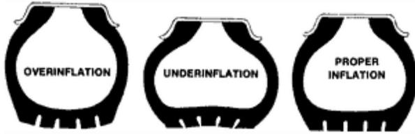
**Overinflated** tires have too much pressure in them and only the center of the tire will grip the road properly and it will wear out more quickly in the center of the tire and will not last as long.
