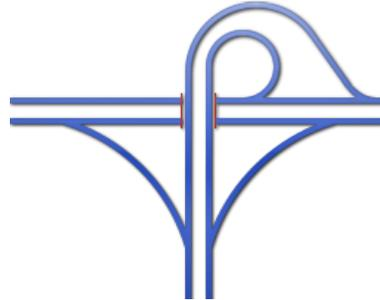
A trumpet interchange is used when a side road forms a “T” intersection with a freeway.
