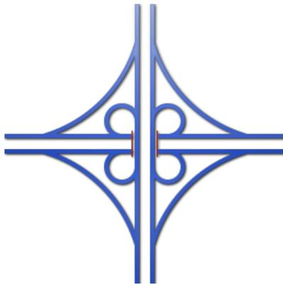
A cloverleaf interchange has multiple entrances and exit ramps that resemble a four-leaf clover. The type of interchange allows driver to go in any of four directions.
